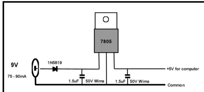
Due to the power consumption being low, the game can be powered by a 9V Alkaline cell which has about a 500mAH capacity or a 9V lithium cell with a 1200mAH capacity. However, in this design, inside the case, there is plenty of room for 6 AAA cells in a holder to significantly increase the running time.
