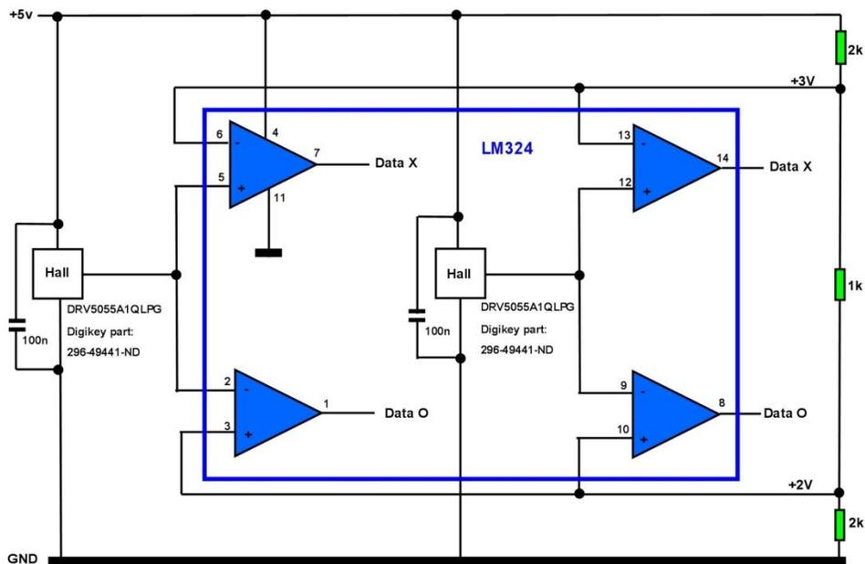
With no applied magnetic field the DC output of the Hall device sits within 70mV of 2.5V
