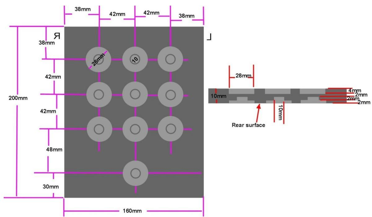
The diagram below, top left, shows the positions of the screw holes that mount the Encoder Board to the bottom of the player panel. These were drilled 8mm into the material and tapped with a 4-40 UNC thread Taper then End tap so as to receive some 4-40 UNC threaded stand offs, of the sort used on computer connectors. These are sold at Jaycar. These allow the Encoder board to be attached and for the Static Computer pcb to be fitted on top of it.
