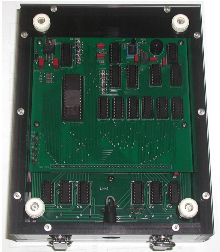
All through hole components are used. Of note there are no Electrolytic Capacitors used in this design, only film types, this makes the circuitry very long lasting.
