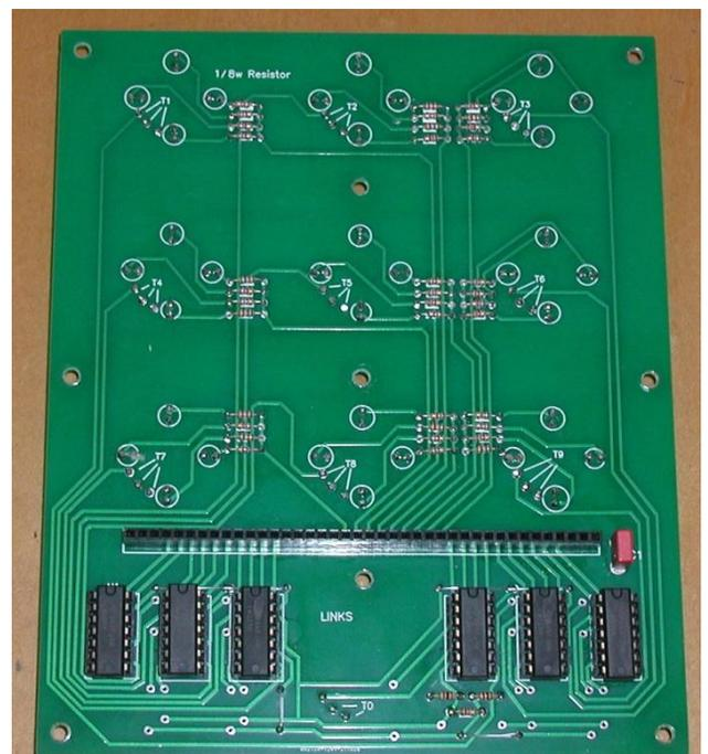
Four LED's on each player board position are used for two reasons. One reason is symmetry and a pleasing appearance, the other is redundancy. If one LED fails (it does happen sometimes) the game can still function normally. Each LED in the group of 4 has its anode connected to +5V and each has a separate cathode resistor. Each LED has around a 1mA operating current, but being Blue LED's, they are quite bright at this low current.
